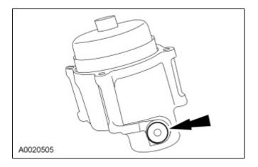
2. Remove the reverse servo spring and check valve.
