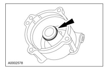
2. Lubricate and install the reverse servo piston and seal assembly.
