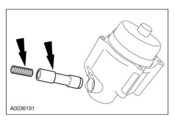
3. WARNING: Follow the specified procedure when using the tool to remove the servo cover. The servo and servo cover are under high spring force and can separate forcefully, which may result in serious personal injury.
