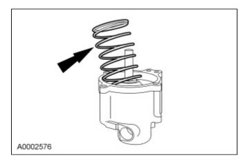
4. WARNING: Follow the specified procedure when using the tool to remove the servo cover. The servo and servo cover are under high spring force and can separate forcefully, which may result in serious personal injury.
