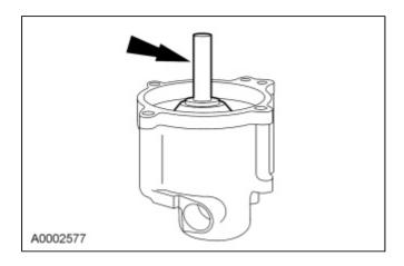
6. Remove and discard the reverse servo piston seal.
