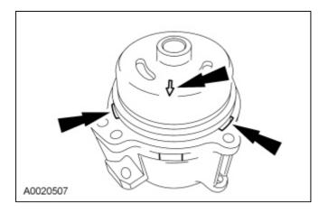
5. Install the reverse servo spring and check valve.
